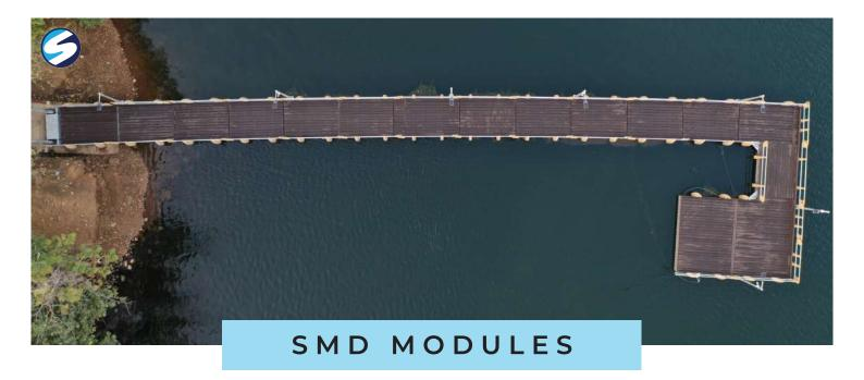
The Superior Modular Dock (SMD) System is made from Rotomoulded Polyethylene modules that are durable, UV stabilised, tough and slip resistant and can be configured into a variety of shapes and applications. It is the main building block of Superior Jetties Floating Platform Systems. These are available in a wide range of sizes - allowing for multiple layouts. These are easily mountable as well as moveable.
